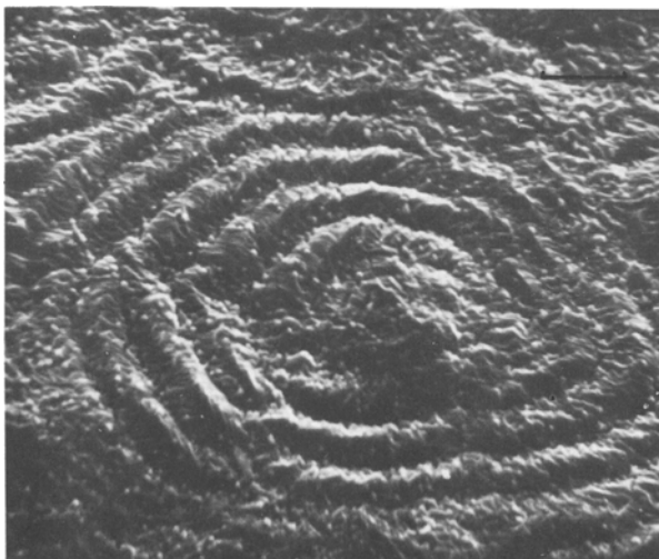
Figure 1 Scanning electron micrograph of an undeformed spherulite of HDPE. The small spheres are artefacts. Scale = 10 \mu\text{m} .
